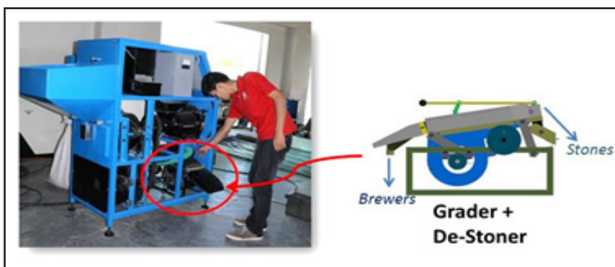
Figure 5. Design of de-stoner and mini-grader of the developed rice mill, 2015
