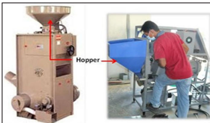
Figure 4. Difference in location of hopper of traditional rice mill (left) as compared with the developed technology (right), 2015
